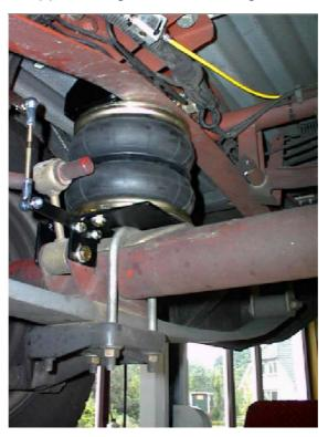
Rotate the bottom plate so that the longitudinal axis is parallel to the top plate. Set the bottom plate so by tightening the M10  $\times$  70 bolt with locking nut Apply now to run a car on height, so the bellows height is 14cm. Right from the bellows, so that is centred and set it down.
